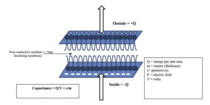
**Figure 2.**Because a cell's diameter is much larger than its membrane thickness, it is reasonable to ignore the curvature of the cell and think of the plasma membrane as a parallel-plate capacitor, where Q is charge per unit area, and capacitance is equal to charge divided by voltage.
